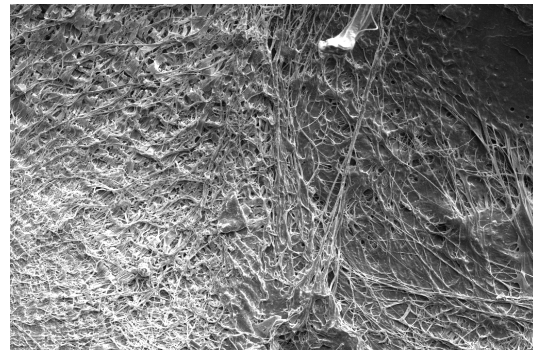
Partial fracture surface of polybutylene tested in fatigue [1]
