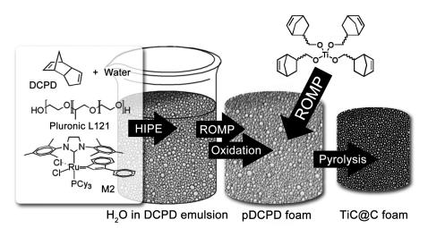
The synthetic route comprised emulsion templating of dicyclopentadiene [3], curing of the emulsion via ROMP, oxidation of the resulting monolith, filling of the pore structures with a Ti-monomer, a second ROMP step, and finally carbonization at  $1400^{\circ}$ C. The resulting conductive TiC foams were shown to be superior cathode materials in Li-O<sub>2</sub> batteries in comparison to similarly prepared carbon foams and TiC nanoparticles.
